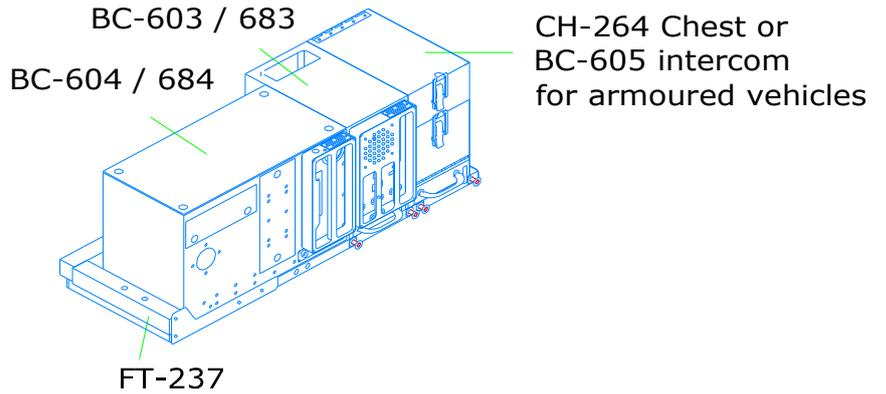
SCR-508 series: for low frequency range, 20-27.9 MHz. Output 30W. 12-24 VDC.
