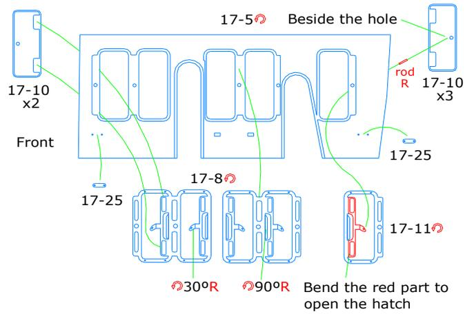
Take attention to the position of the parts 17-6 and 17-10: there are 2 hatches that open forward, and 4 hatches that open backward
