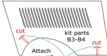
Cut the support of the kit part A51 and fit the triangle here
